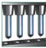
1 Preform Injection Station
